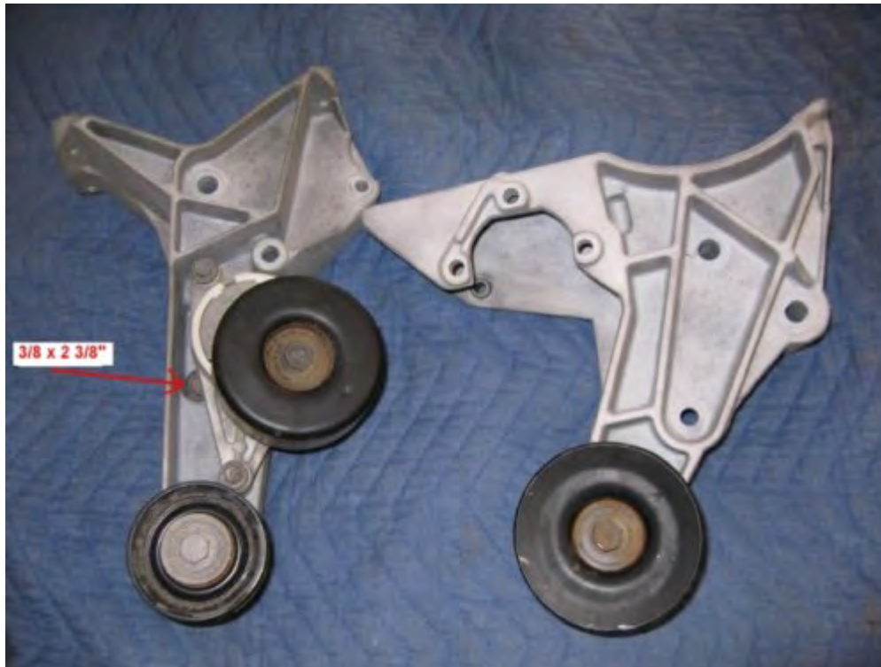
Figure 5B. This bolt is not used on the 351W. The power steering/A/C compressor bracket is shown on the right (in this view rotated 90 degrees counterclockwise from its mounted position). These represent all the idler pulleys and can be rebuilt with new bearings if your serpentine setup came from a high-mileage engine.
