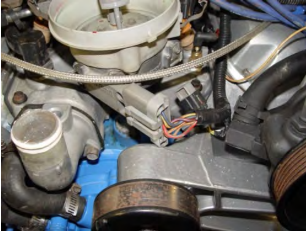
Figure 5D. The TFI module can interfere with the serpentine bracket. Solutions include clearancing the bracket slightly or installing the distributor slightly counterclockwise (maybe about 1 tooth over).
