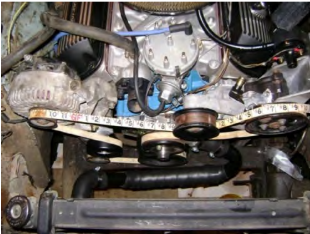
Figure 13B. Method for measuring the belt size for conversion without A/C compressor.
