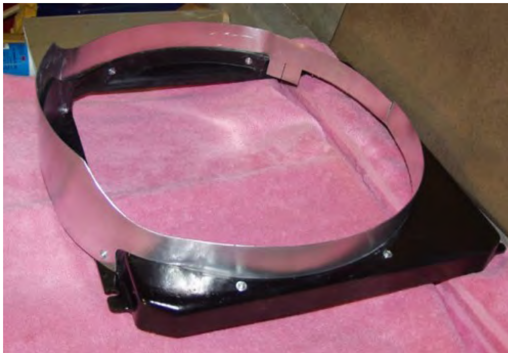
Figure 9B. The finished shroud wraps around the existing factory shroud and extends it about 2 inches.
