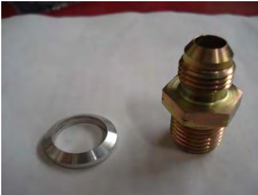
Figure 7B. Lee Manufacturing power steering pump metric 16mm x 1.5-to-AN-hose adapter. The corresponding Russells fitting use a rubber O-ring instead of the flare fitting with metal washer.
