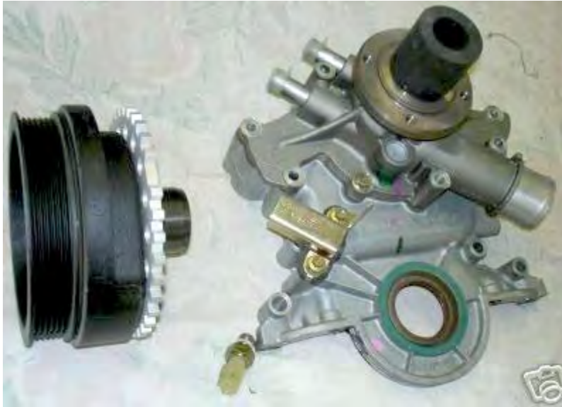
Figure 3a. Typical 5.0 Explorer timing cover and integral balancer-crank pulley. You will want to substitute the gold piece in this picture (crank position sensor, which you will not need) with a simple timing pointer (see Figure 4).
