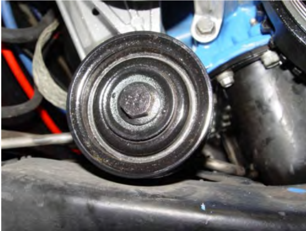
Figure 5C. The lower passenger side belt idler pulley can be very close to the frame. There should be a minimum of 1 inch clearance. If it is less, the easiest option is to raise the engine with shims between the motor mount and block.
