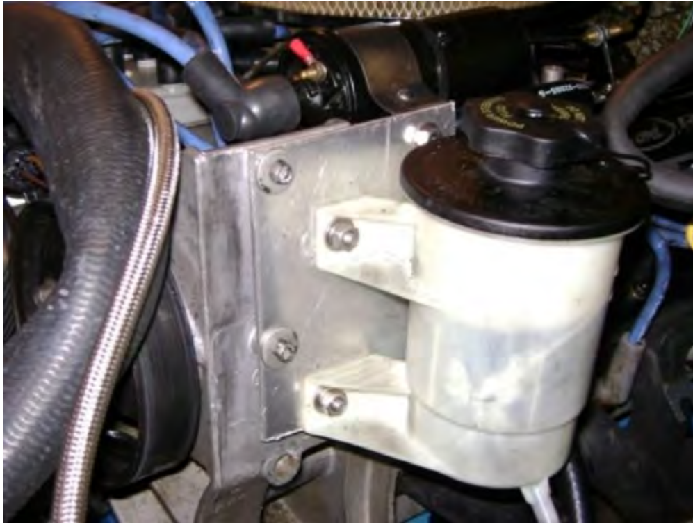
Figure 10B. If you are running a carbureted engine, here is the coil attachment for a standard cylindrical coil. Simply attach it to the top of the power steering reservoir offset plate.
