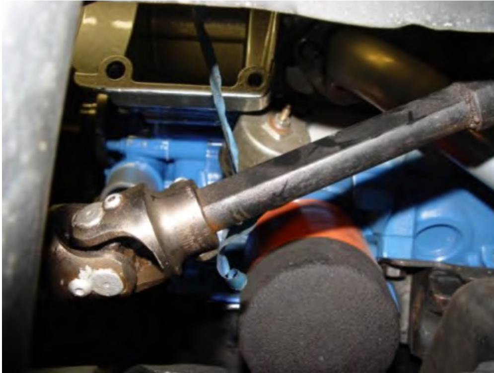
Figure 5E. View with the A/C compressor not mounted in order to show the oil pressure sensor to bracket clearance. In most cases, clocking the oil pressure sensor extension housing provides clearance.
