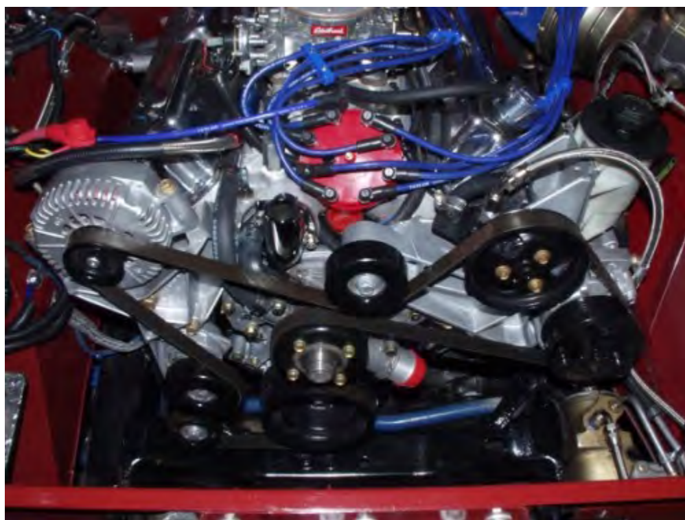
Figure 1. Example of the Explorer 5.0 serpentine belt system installed in an early Bronco. Note that all the accessories are mounted high, instead of being buried in the dark reaches of the engine bay. This particular example is on a 5.0 Ford Racing crate motor. (The A/C compressor bolts are close to the inner fender, so keep that in mind; you may want to have the compressor in place before bolting the bracket up. Access holes in the inner fender, filled with rubber plugs would be nice so you can remove it later if need be.)
