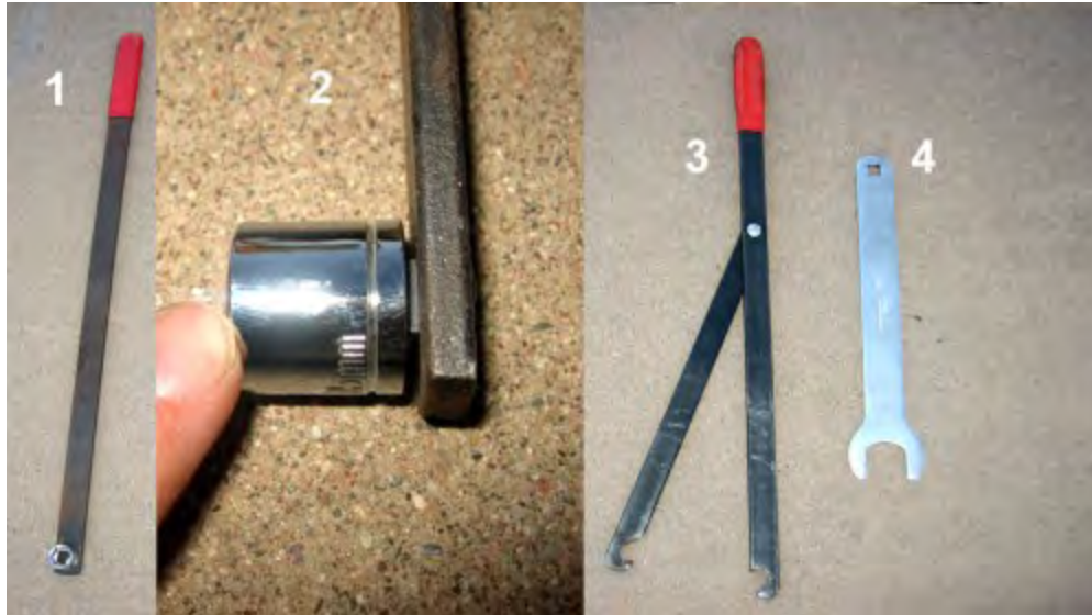
Figure 8. Tools made for work on the pulley tensioner and fan clutch assembly. Most of these can be substituted with ingenuity, but #4 is especially nice if you have access to one. (1) tensioner wrench and (2) narrow socket used to release tension on the serpentine belt tensioner so the serpentine belt can be removed (Performance Tools W84010). The scissors-shaped tool (3, K-D Tools 3471) is designed tool to grab 2 of the 4 water pump pulley bolts so the fan/clutch assembly can be removed more easily. And the Fan clutch wrench (4, Performance Tools W80585) is used to loosen the nut that holds the clutch assembly onto the water pump.
