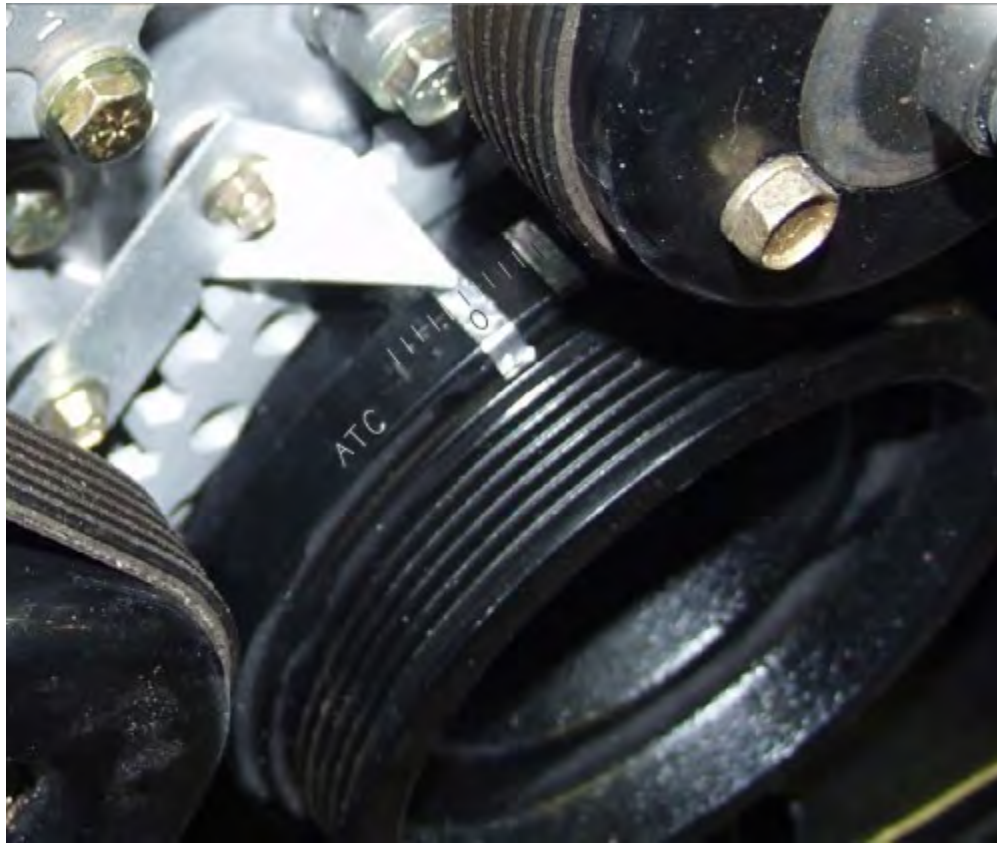
Figure 4B. Here is the timing pointer location, and an example of one that you can make up. Start out with a piece of cardboard and fab it to fit before cutting metal. A piece of aluminum or sheet metal will do fine. The timing marks are not easy to find. Worse still, there is a big groove in the damper that looks like a timing mark but is not. So look carefully.
