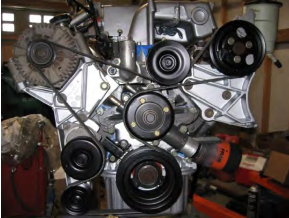
Figure 13A. Photo of belt routing without A/C compressor.
