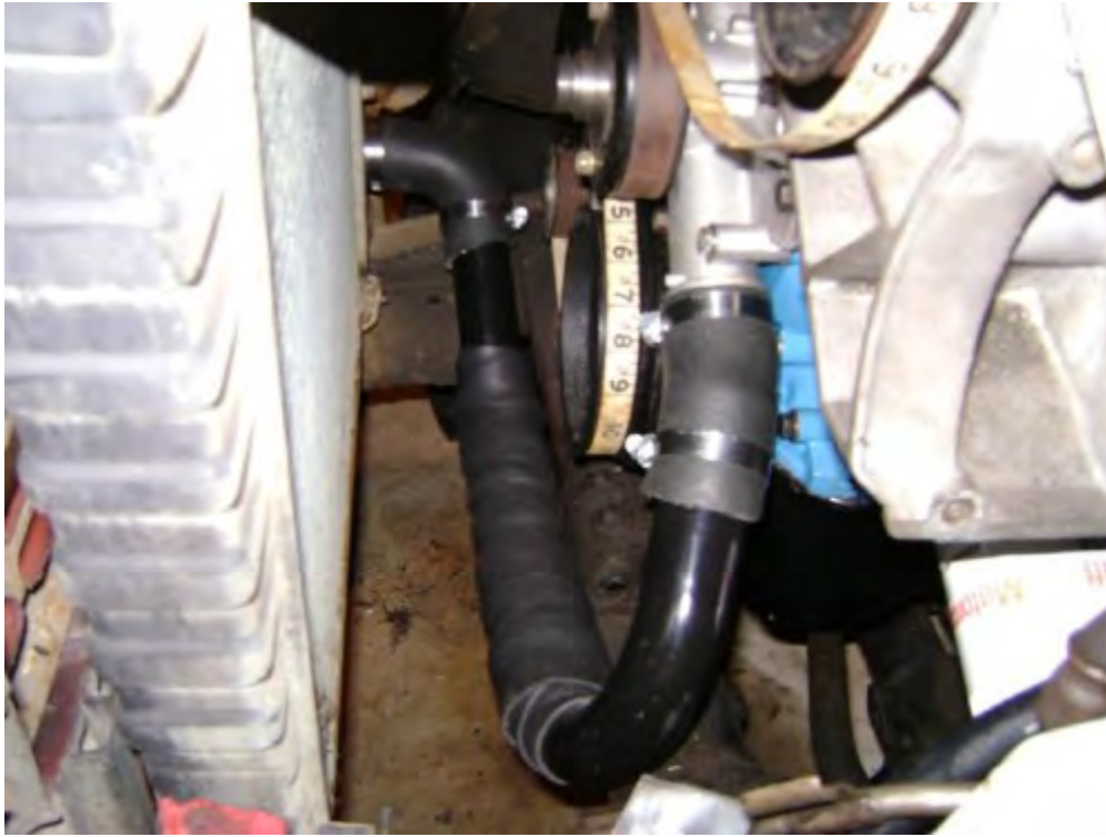
Figure 9C. Crossover hose option for use if you are running an original Bronco radiator instead of the 5.0 ("reversed inlet/outlet) radiator.
