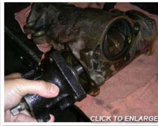
Photo 8: Keep the splines pointed toward the sector shaft bore as you install the valve and worm assembly.
