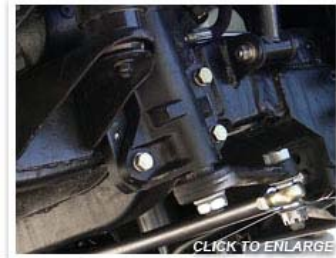
Photo 13: The Rockcrawler Box Adapter Plate makes the install an easy bolt-on.
