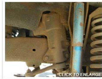
Photo 1: The 4X4 box mounts to the outside of the frame on 78/79 Broncos and 76-79 F150 4X4 pickups.
