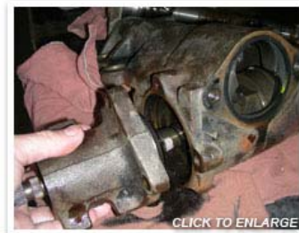
Photo 6: Make sure the input shaft and valve housing do not spin as you pull the valve/worm assembly out of the gearbox housing.
