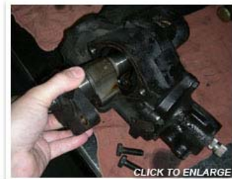
Photo 5: Remove the sector shaft from each gearbox.
