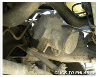
Photo 2: The 4X2 box is found on the inside of the frame rail on a wide variety of Ford trucks from the 80's through the mid-90's.
