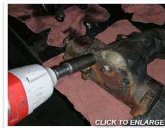
Photo 9: A pneumatic or electric impact wrench makes quick work of the disassembly and assembly.
