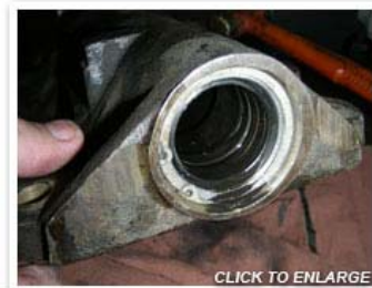
Photo 11: The sector shaft seals are a common leakage point, but they're easy to get to.
