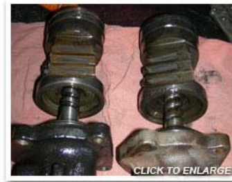
Photo 7: Note the different direction of the worm spiral from each gearbox.
