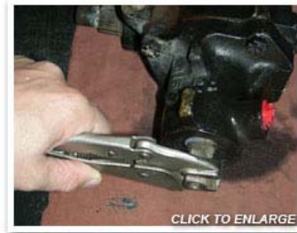
Photo 3: Be careful not to damage the splines when using vise grips to rotate the input shaft.
