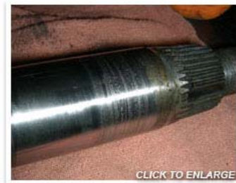
Photo 9: The seal surface on this sector shaft is showing some wear and should be polished prior to reinstallation.
