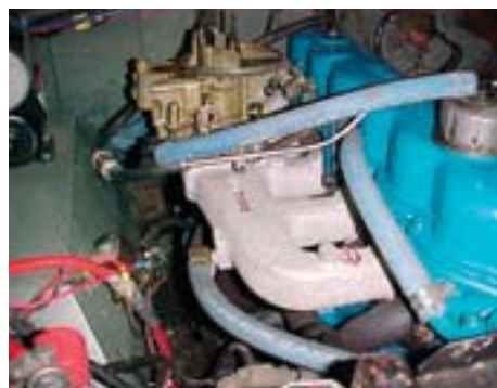
A view of the Clifford 6 into 2 header.
