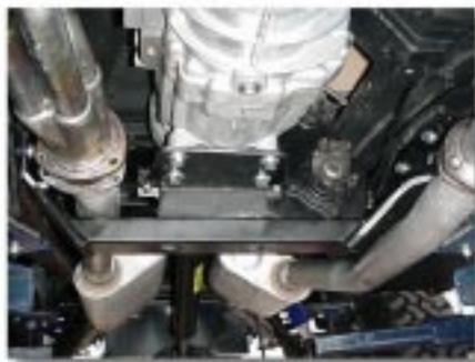
The new crossmember is a tight fit between the transfer case and transmission. A notch has been cut in the crossmember for clearance of the Dana 20 front output retainer bolt. This notch is necessary on applications using the stock transfer case rotation.
