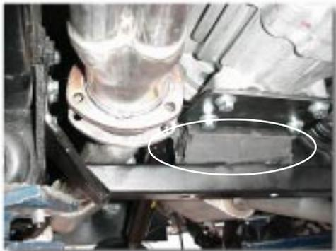
The crossmember can now be fitted to the rubber mount and the frame rails. The driver's side exhaust should fit under the crossmember and the passenger side exhaust should fit inside the crossmember. Depending on the exhaust configuration in your vehicle, you may be required to do so modifications to the exhaust for proper fit.
